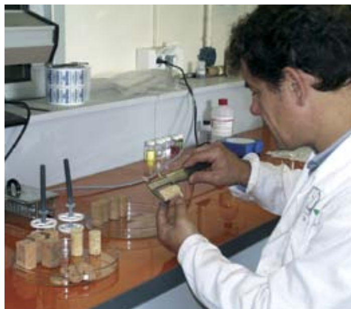
■ Photo 2: Dimensional variation measurements on cork closures.
